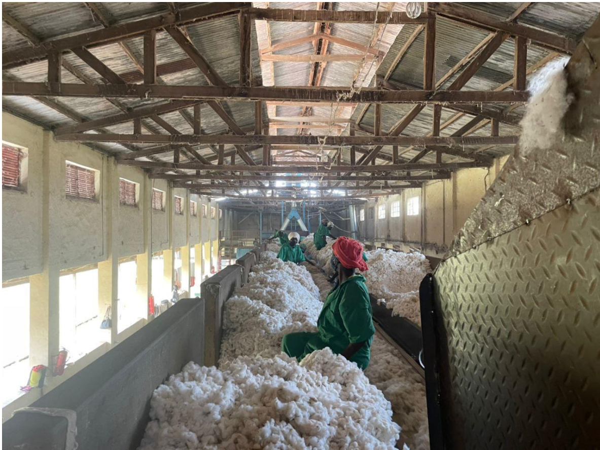
Kitgum ginning hall, the cotton on platform about to be ginned for the lint and seed to be separated.
